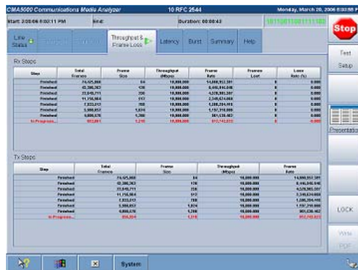
Fig.2: Automated RFC 2544 application for quick verification of network performance. All details results provided in comprehensive reports.
