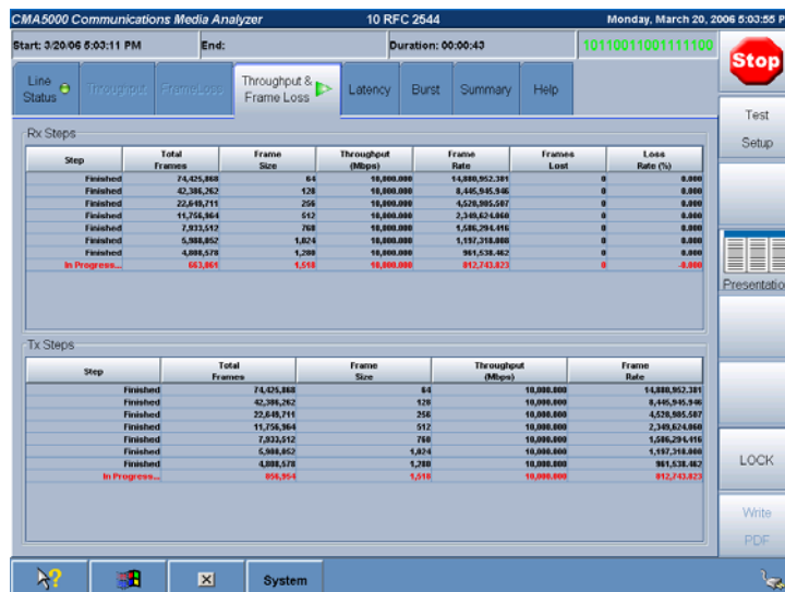
Fig.7: Automated RFC 2544 application for quick verification of network performance. All details results provided in comprehensive reports.
